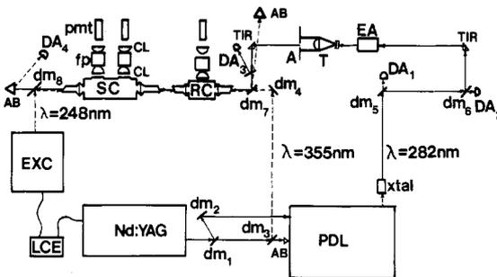
**Figure 2.** Optical layout for PF-LIF HONO detection system: A, aperture; AB, absorption beam dump; CL, fluorescence collection lens; DA, laser diode; DM, dichroic mirror; EA, laser energy attenuator; EXC, excimer laser; FP, optical filter pack; LCE, laser coupling electronics; PMT, photomultiplier tube; PDL, pulse dye laser; RC, reference cell; SC, sampling chamber; T, telescope; TIR, beam steering prism; XTAL, frequency doubling crystal.
