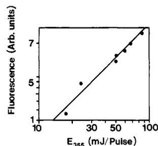
**Figure 6.** Photolysis laser energy scaling of PF-LIF HONO fluorescence signal (laboratory results)—nonforced least-squares fit of data.
