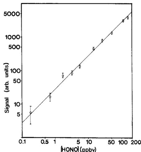
**Figure 11.** Calibration plot for PF-LIF HONO detection system (laboratory results)—nonforced least-squares fit of data.
