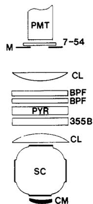
**Figure 4.** Detection optics and filter pack for PF-LIF HONO detection system: 7-54, colored glass filter; 355B, 355-nm blocking filter; BPF, band pass filter (309-nm); CL, fluorescence collection lens; CM, fluorescence collection mirror; M, PMT mask; PMT, photomultiplier tube; PYR, pyridine solution filter; SC, sampling chamber.
