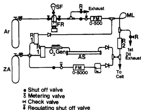
**Figure 5.** Schematic diagram of HONO flow calibration system: AR, argon cylinder; AS, absorption cell; FM, linear mass flowmeter; FR, HONO flow reactor; ML, mixing loop; R2, Teflon rotameter; SF, sodium nitrite solution; ZA, zero air.
