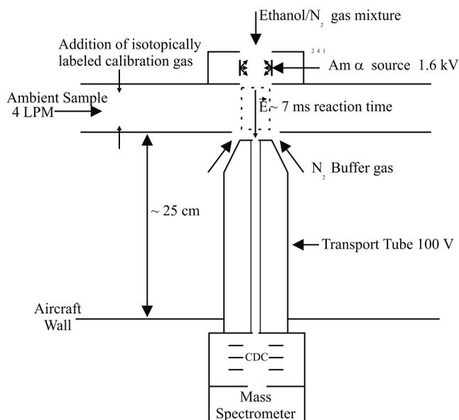
**Figure 1.** Diagram of the ion-molecule reactor used in this study.
